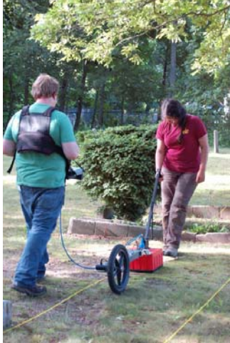
Ground penetrating radar survey
