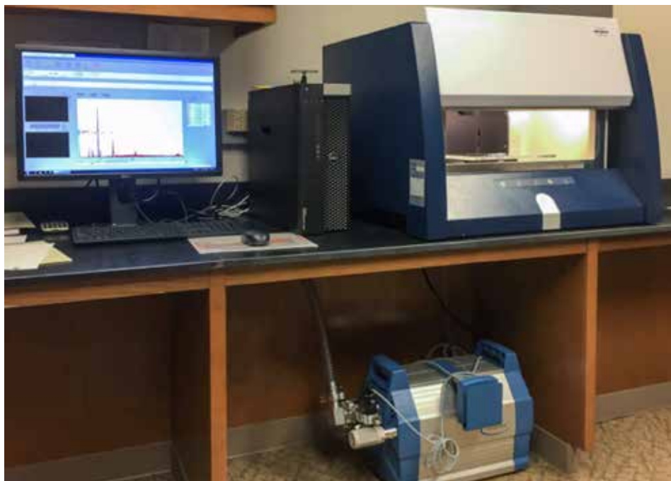
Meet the Bruker M4 Tornado, ready for business on the Keck lab bench.
